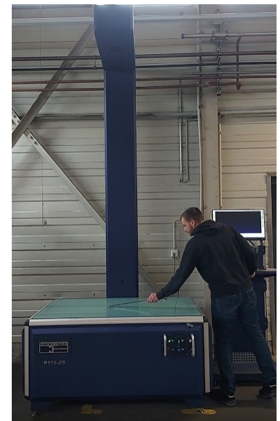
Figure 2: Metal part being measured on Planar machine at BVS
